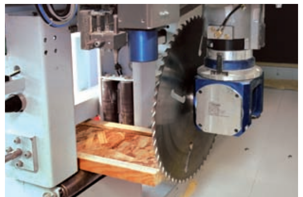
Flexibility to handle I-Joist, LSL, LVL and solid sawn lumber
