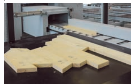
Cross transfer of finished parts.
