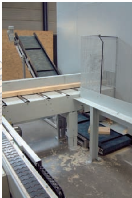
Available conveyor systems for small part retrieval and and waste removal (optional).
