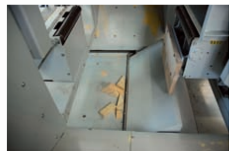
Automatic processed part sortation for pieces smaller than 160mm.
