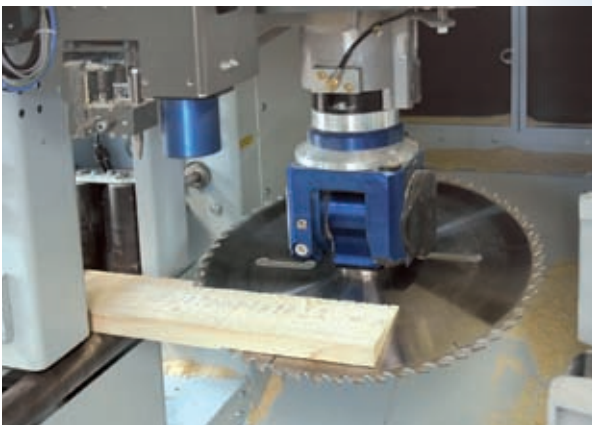
Rip and scarf cuts, beveling and slotting (0-90 degree rotating angle)
